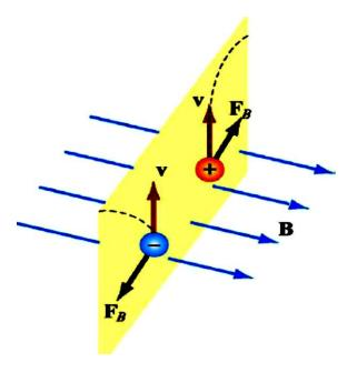
When a charge particle moving with a constant velocity **(u)** and entered to a region contain a constant uniform magnetic field is experienced by a force due to the magnetic field and make it to move in a circular motion as shown below:
