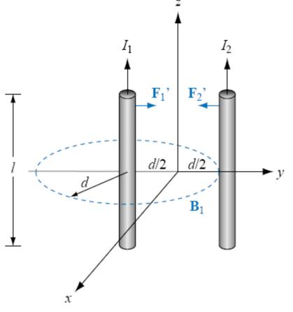
Then the magnetic force ( $F_2$ ) exerted on a length (L) of wire carrying current ( $I_2$ ) due to its presence in field ( $B_1$ ) may be obtained by applying the following equation:
