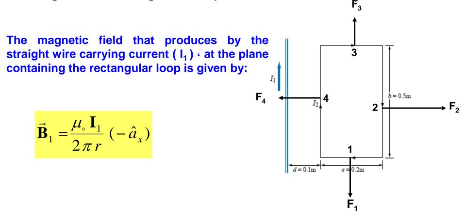
Then the magnetic force exerted by this field on the individual dimensions of the loop is calculated as:
